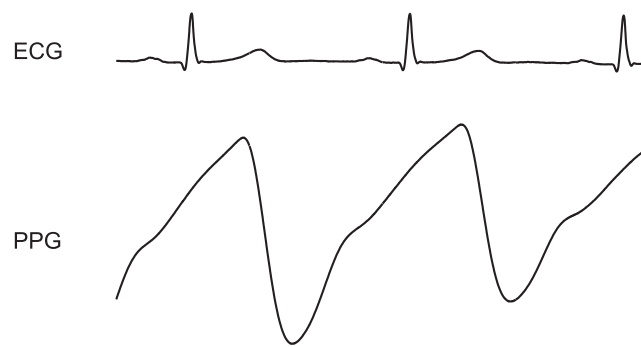
Figure 1. The pulsatile (AC) component of the PPG signal and corresponding electrocardiogram (ECG). The AC component is actually superimposed on a much larger quasi-DC component that relates to the tissues and to the average blood volume within the sample. It represents the increased light attenuation associated with the increase in microvascular blood volume with each heartbeat. In practice, the PPG waveform is often inverted.
