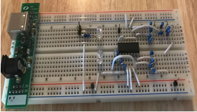
Figure 5. The Implemented PPG device with a modulated light source (ML-PPG design)
